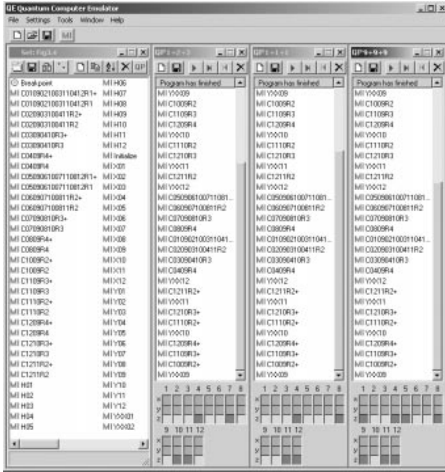
Figure 12. QCE implementation of the quantum network of Fig. 11 for adding three quantum registers of four qubits each. QPs (from left to right) compute 1+2+3 , 1+1+1 , and 9+9+9 \pmod{16} . Not shown are the MIs that set the initial values of the three four-qubit registers.
