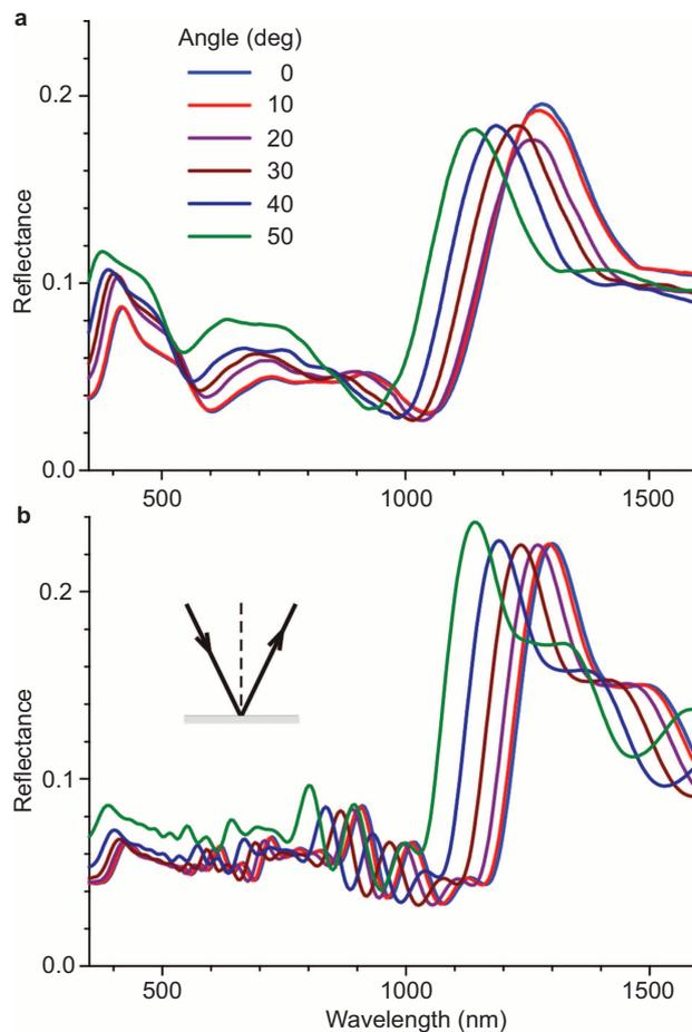
**Figure 5** Angle-dependent reflectance spectra. (a) Averaged spectra calculated for 36 lanes of the transmission electron micrograph of Figure 2f, for angles of incidence  $0^\circ$ – $50^\circ$ . (b) Reflectance spectra measured for each angle of incidence at the mirror angle.
