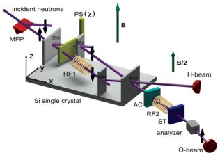
Fig. 14. A single-neutron interferometry experiment for the observation of interference between the phases induced by a phase shifter (PS) and by two RF fields.<sup>59</sup> BS0,...,BS3: beam splitters; MFP: magnetic field prism; B = Be,: constant magnetic field; PS: phase shifter; RF1, RF2: radio-frequency spin-flippers; AC: accelerator coils; ST: spin turner.
