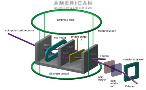
Fig. 10. Diagram of the single-neutron interferometry experiment to observe correlations that cannot be accounted for by a quantum system in the product state, see also Figure 1 in Ref. [53]. BS0,...,BS3: beam splitters. The combination of the mu-metal spin turner, phase shifter, and spin rotator allow the independent manipulation of the neutron's spatial and magnetic degrees of freedom.
