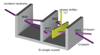
**Fig. 1.** Picture of the perfect crystal neutron interferometer.<sup>12</sup> BS0,...,BS3: beam splitters; phase shifter: aluminum foil; neutrons that are transmitted by BS1 or BS2 leave the interferometer and do not contribute to the interference signal. Detectors count the number of neutrons in the O- and H-beam.
