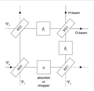
**Fig. 8.** Diagram of the single-neutron interferometry experiment with a stochastic or deterministic absorber.<sup>12</sup> BS0,...,BS3: beam splitters;  $\phi_0$ , and  $\phi_1$ : phase shifters. Neutrons pass through the stochastic or deterministic absorber with probability *a*.
