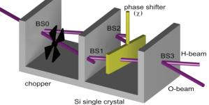
Fig. 7. Diagram of the single-neutron interferometry experiment with a stochastic (top) and deterministic (bottom) absorber.
