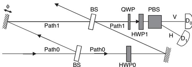
**Fig. 1.** Schematic diagram of the experimental setup for the quantum eraser experiment with photons studied in Ref. [8]. BS: beam splitter; PBS: polarizing beam splitter; HWP0 and HWP1: half-wave plates; QWP: quarter-wave plate;  $D_0$ ,  $D_1$ : detectors;  $\phi$ : phase shift introduced in Path1.
